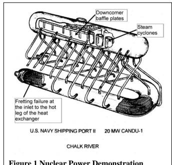
Figure 1 Nuclear Power Demonstration (NPD) illustration
