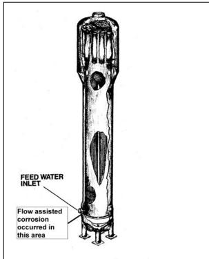
Figure 3 Pickering A Steam Generator.
